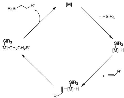
**Scheme 2.** Silyl Migration Mechanism for Hydrosilation and Dehydrogenative Silylation of Olefins
