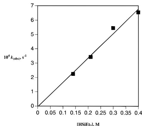
**Figure 1.** A plot for  $k_{\text{obs}}$  vs  $[\text{HSiEt}_3]$  for the reaction of [(phen)Pd(SiEt<sub>3</sub>)(H<sub>2</sub>C=CH-*t*-Bu)]<sup>+</sup> (**4b**) with HSiEt<sub>3</sub> to form **2a** and *t*-BuCH<sub>2</sub>-CH<sub>2</sub>SiEt<sub>3</sub> (-38 °C; [**4b**] = 0.014 M;  $k_{\text{obs}}$  = 1.7 × 10<sup>-3</sup> s<sup>-1</sup> [HSiEt<sub>3</sub>]).
